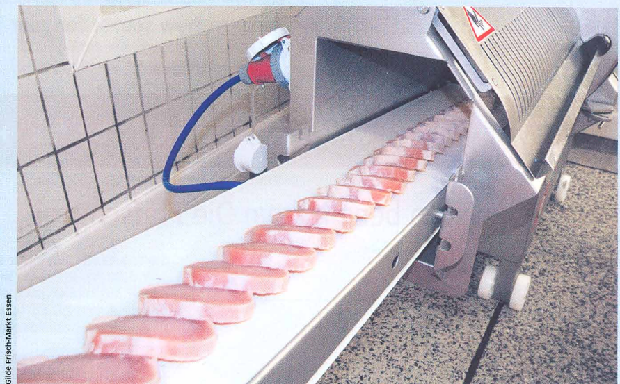
With the Puma, slices are cut in uniform portions and can be deposited in packages continually or shingled.
