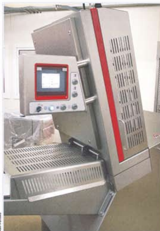
High speed: Up to 1,760 cut-off sections per minute can be processed on the Divider type 440.
