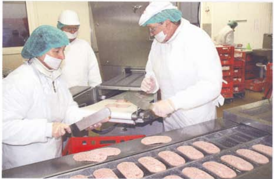
With the Divider 440, cutting and depositing is simultaneous, i.e. in one single operating step.
